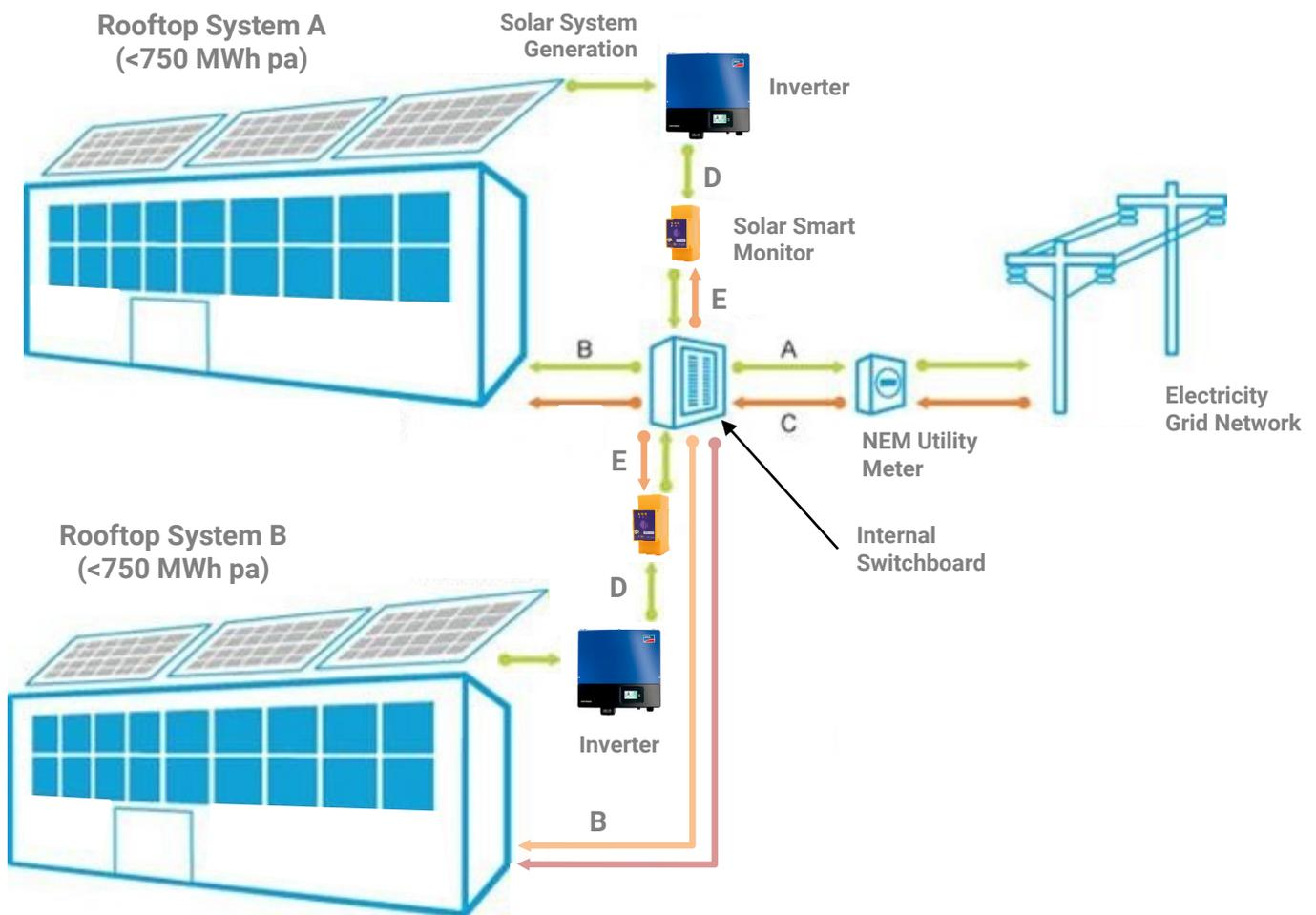
Diagram 1: Solar power station energy flows. Solar Smart Monitor measures total solar electricity generation (less any AUX consumption). A = net energy exported via NEM connected utility meter. B = solar energy consumed on site. C = energy imported from the grid. D = energy production from rooftop power station, E = energy consumed by solar power station.
